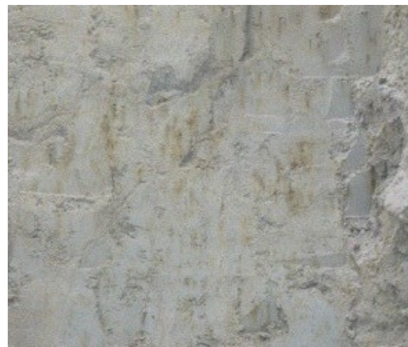
Figure 23 A mottled clay subsoil, where the main soil colour is grey and there are faint pale-yellow mottles
