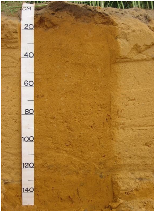
Figure 12 Profile of a gradational soil with sandy loam topsoil grading to sandy light clay subsoil
