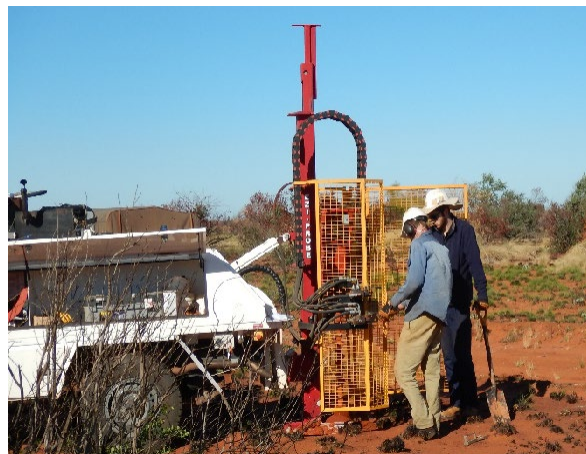
Figure 4 Soil samples being collected using a drill rig
